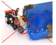
Cables with open ports or bare parts have to be cut so that no bare wires are visible. Cut the wire as close as possible to the battery.
