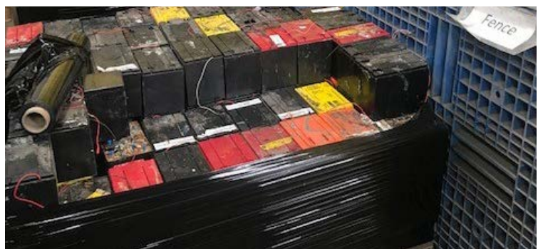
Fence Batteries shrink-wrapped on wooden pallets
